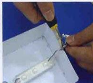
5, Cut off the odds and fix wires
