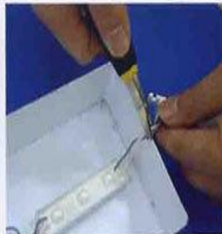
5, Cut off the odds and fix wires
